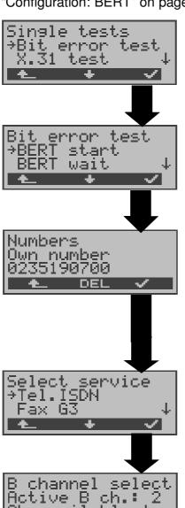
In the Single tests menu, use the  $< \downarrow >$  to select **Bit** error test.
