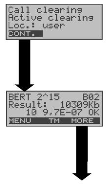
After the test time is over, the ARGUS will display the cause and the location which initiated the disconnect.
